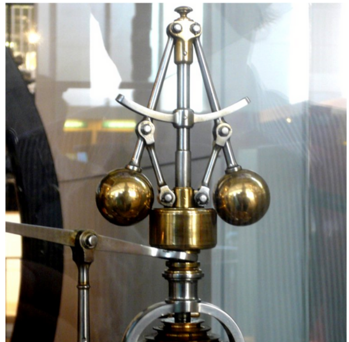
Centrifugal Governor at the Science Museum London. picture by Mirko Junge. See e.g. https://www.reddit.com/r/steamporn/comments/2c8kk5/centrifugal_governor_at_the_science_museum_london/
